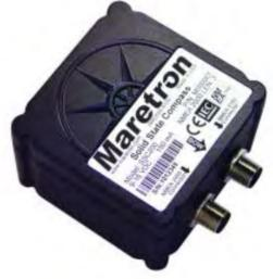
Magnetic compass as the primary means of determining heading. The heading data is used to calculate wind direction, current data, and VMC performance data. A 3D compass also provides data to calculate precise pitch, heel, and turn rate.
